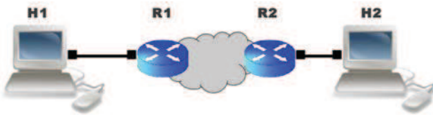
Figure 2. Basic network topology with 2 hosts and 2 routers
